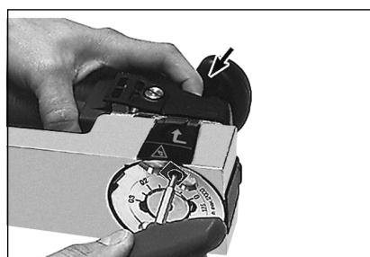
Press the locking button (2) up to the stop and keep pressed.
